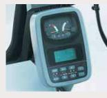
The LCD multi-display shows a malfunction log (including fuel, hydraulic oil, cooling water, etc.) for 16 items, and its self-diagnostic function monitors a total of 41 items, including electrical malfunctions involving solenoid valves, sensors, etc.
